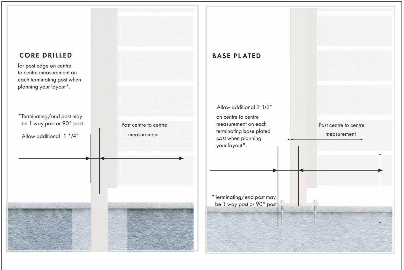
**5** Determine post positions. For simplicity, calculate post positions from centre of post to centre of post. Recommended that post centres do not exceed , in areas of high wind, consider restricted span widths.
