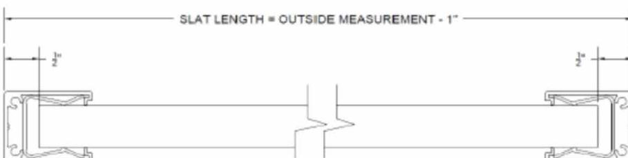
**TO DETERMINE SLAT LENGTH, DEDUCT 1" FROM THE OVERALL WIDTH OF THE PANEL, AS SHOWN IN THE ADJACENT DIAGRAM.**
