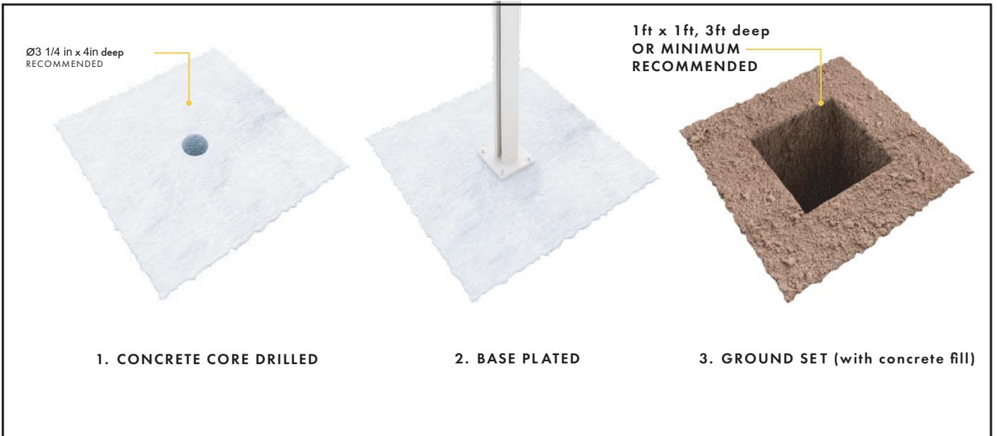
**3** Determine how posts are to be installed:
