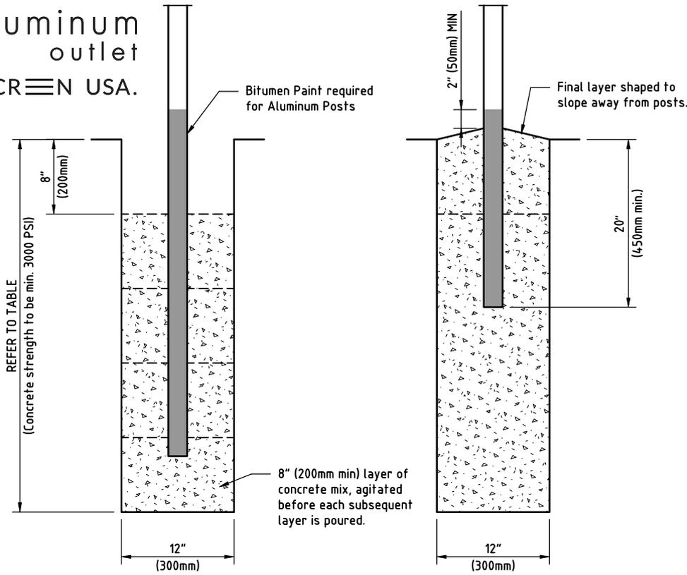
**POST CAST INTO FOOTING DETAIL**
