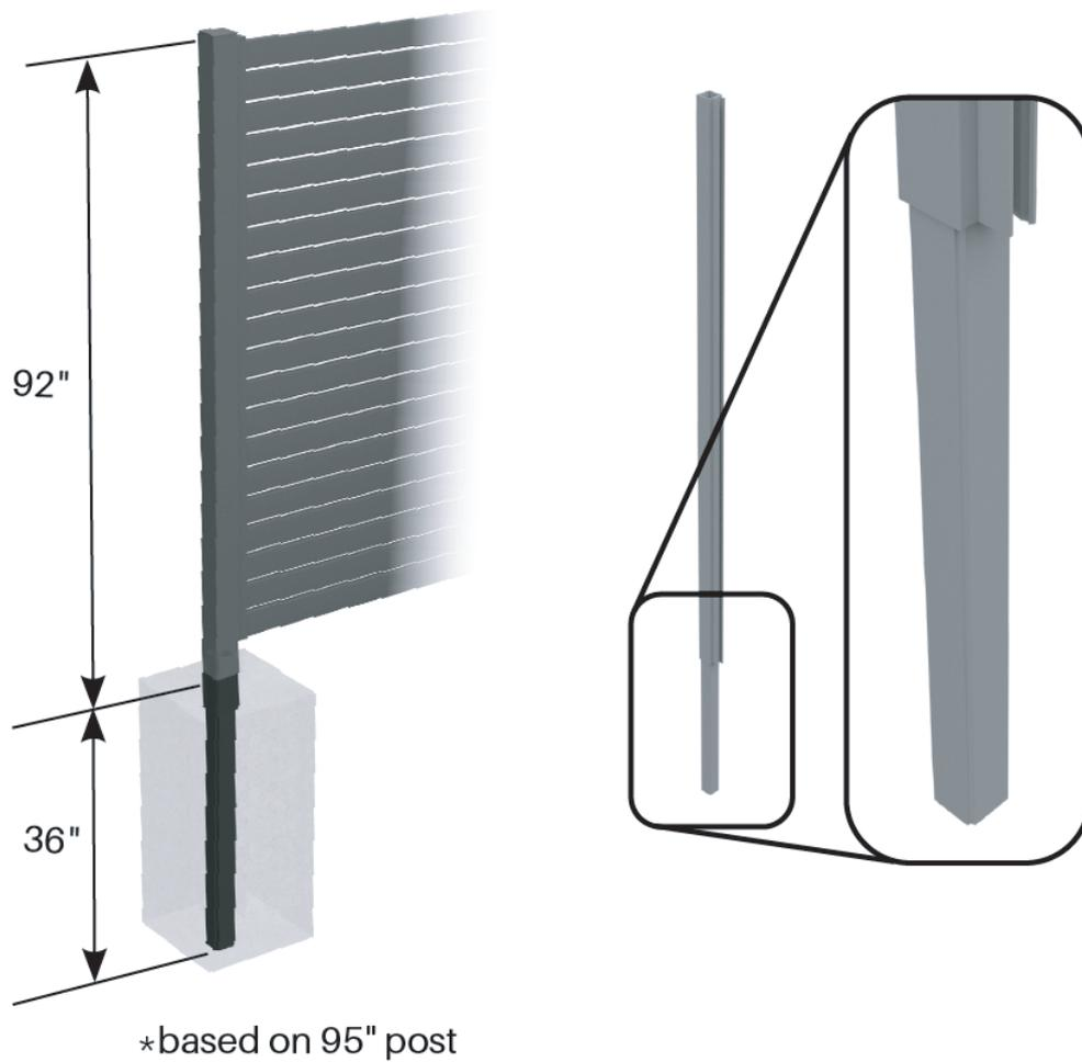
For use when posts need to go into ground more than 24" or fence higher than 6' (will also require side frame).
