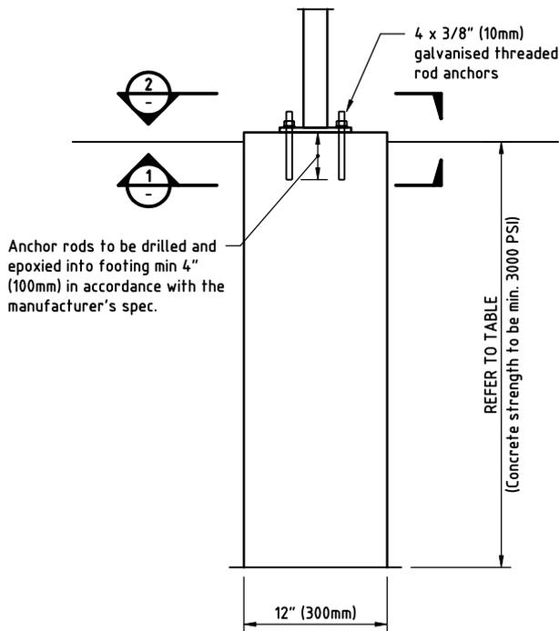
**POST INSTALLED ON TOP OF FOOTING DETAIL**
